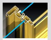
A key feature of the 541 is the clean flydoor installation. The screens have a snap-on interlock that nest into the interlock on the glass door. Detail above also shows the optional stile closer:
